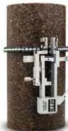
Model 632.92H-05 Extensometer on Marble Core Specimen
