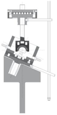
Cross-section schematic showing the pin bearing assembly housed within the inclined mounting block, which rotates to provide the biaxial walking motion. Alternate specimen mounting where the ball is attached to the top fixturing can be provided.
